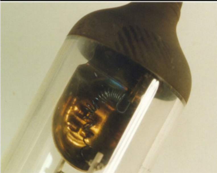
(Headlamp filament damage)
