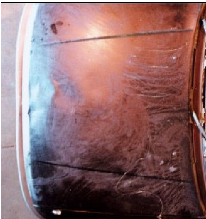
(Overhead view of dented bumper, leading edge and bonnet from pedestrian impact)
