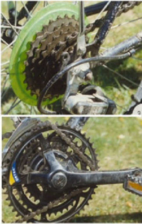
(Top - bicycle rear cassette and derailleur detail. Bottom - bicycle chain and chain-ring detail)
